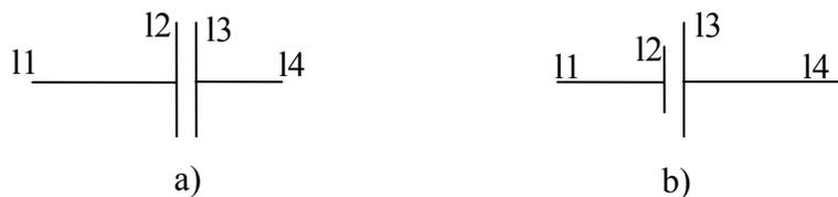
**Figure 7.12 a) Battery symbol. b) Capacitor symbol**
