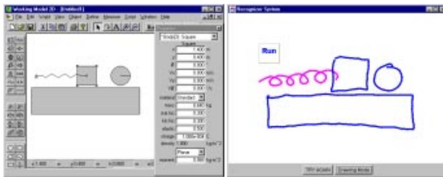
Figure 1: **A block and spring constructed in CAD and in ASSISTANCE.** In the CAD tool, the designer selects components from templates and specifies parameters. In ASSISTANCE the designer sketches the block and spring and says “the block pushes the ball.” From this description the system generates a simple causal model in which the spring causes the block to move and that in turn causes the ball to move.
