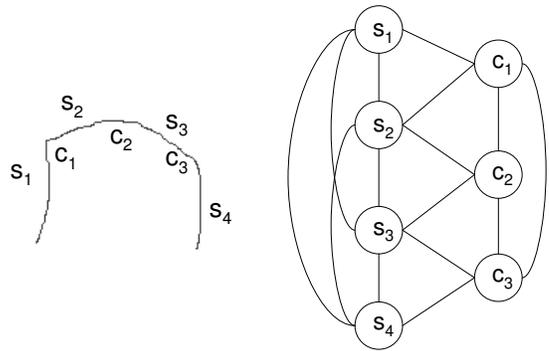
Figure 2: A stroke and its corresponding graph. Possible corners are labeled  $c_1$ ,  $c_2$ , and  $c_3$ . Areas between the possible corners are labeled  $s_1, s_2, s_3$ , and  $s_4$ . Possible corners are found by selecting areas of the stroke with a direction change above a threshold.
